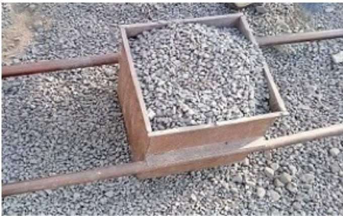
Figure A8: Aggregate & sand measuring box
